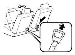
After exiting the vehicle, return the seatback to its upright position.
